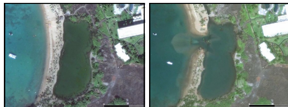
Above: Satellite images show tsunami damage to the rock wall on the island of Hawaii. The left image was taken November 10, 2010; the right, March 11, 2011. Credit: U.S. Army Corps of Engineers Public Notice
